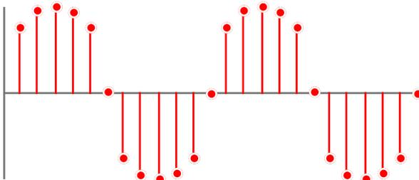
As you can see from above, the information between the samples is lost. The lower the sampling rate the more information is lost. This introduces noise into the signal and reduces the range of audio frequencies that can be represented by the samples, so it is desirable to use a high sampling rate.
