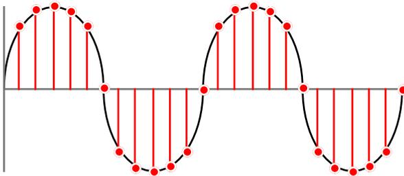
After sampling, the sound wave is represented by a series of discrete samples:
