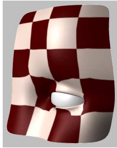
Flat projection converted to UVW mapping. The texture is distorted where areas of high point density meet areas of low point density
