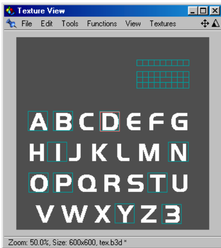
Texture View: the texture is the alphabet with its UV mesh edited so that 'BODYPAINT 3D' appears in the Perspective View. At the top right you can see the 'unused' UV polys.
