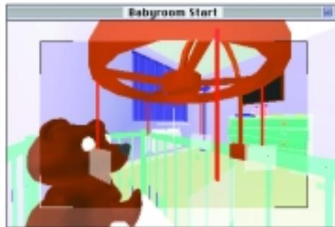
For the final calculation, modify the total duration of the animation by typing in **5 seconds**. Note that all of the path's modifications, the camera behavior, the length of the duration and the number of images per second take place in real time in the preview window.
