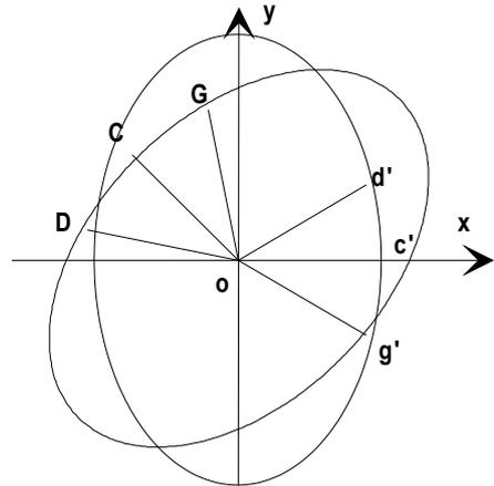
$$\begin{aligned} xG &= d3g \cos ( \text{betag}' + \alpha ) + x0 \\ yG &= d3g \sin ( \text{betag}' + \alpha ) + y0 \\ zG &= zg' + z0 \quad \text{et,} \\ xD &= d3d \cos ( \text{betad}' + \alpha ) + x0 \\ yD &= d3d \sin ( \text{betad}' + \alpha ) + y0 \\ zD &= zd' + z0 \end{aligned}$$
