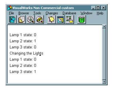
• What happens if we break the dependency on one of the lamp? Let us remove the 2<sup>nd</sup> lamp's dependency on 3<sup>rd</sup> lamp from the ordered collection. Notice that when the 3<sup>rd</sup> lamp turns on the 2<sup>nd</sup> lamp never turns off.
