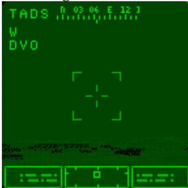
The TADS page relays information from your optical sensors to an MFD. To cycle between the available cameras, you may click on the selected camera display (either DVO, FLIR, or DTV). To pan the camera, move your mouse to the edge of the display and left click using your mouse. You can zoom the cameras in or out using the Plus and Minus keys on the numeric keypad.
