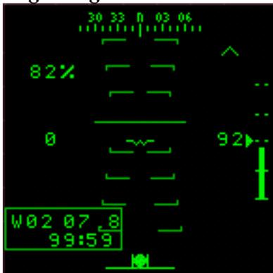
The Flight page repeats information from your IHADSS to an MFD page. Included are a compass, pitch ladder, torque indicator, waypoint information, radar altimeter, and a slip ball.
