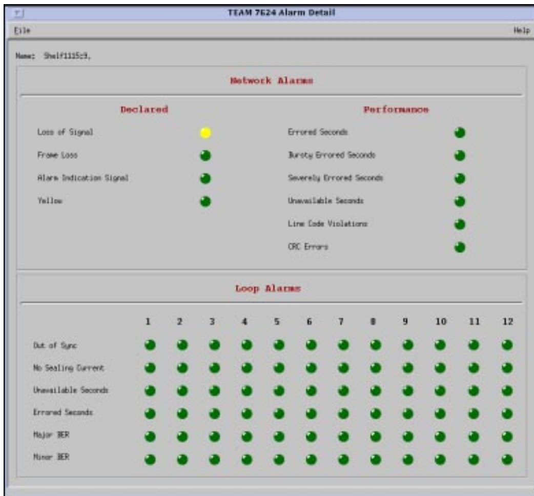
Figure 2-7 Alarm Detail Screen
