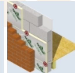
Boards are installed as work proceeds
