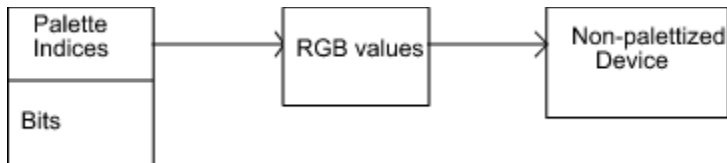
Figure 7. Using StretchDIBits with DIB_PAL_COLORS to draw on a non-palettized device DC.
