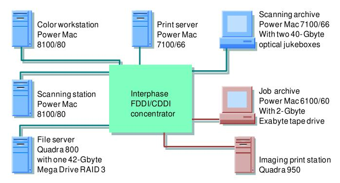
This is a simplified view of Quebecor's network. (There are many more workstations than pictured.) Each Mac server and client has the appropriate FDDI or CDDI client cards. These cards are responsible for boosting transmission speeds to a point that makes the network viable for the movement of large graphics. files.
