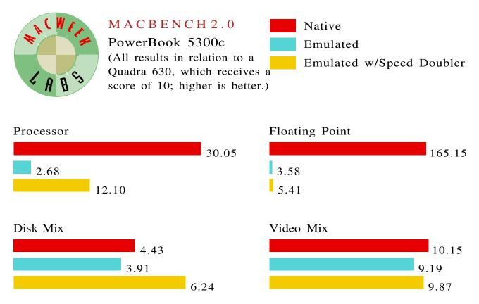
All tests were performed on a PowerBook 5300c with 24 Mbytes of RAM running System 7.5.2. All extensions, AppleTalk and virtual memory were off, and the unit was in full-power mode (plugged in, with no sleep or CPU rest).
