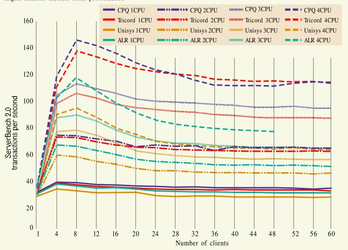
The ServerBench 2.0 System test stresses all facets of the server, from disk to network to processor bus. Despite repeated attempts, however, PC Week Labs was unable to complete the four-processor System test on the ALR Q-4SMP server.
