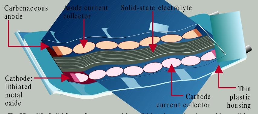
The Ultralife Solid State System combines lithium-ion technology with a solid polymer electrolyte for a thin, flexible, lightweight, and high-energy-density battery that can conform to almost any shape.
