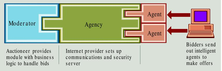
IBM is demonstrating an Internet-based server system, built with Object REXX, that integrates three parts: an infrastructure, called an agency; an application server module, called a moderator; and intelligent agents sent out by bidders.
