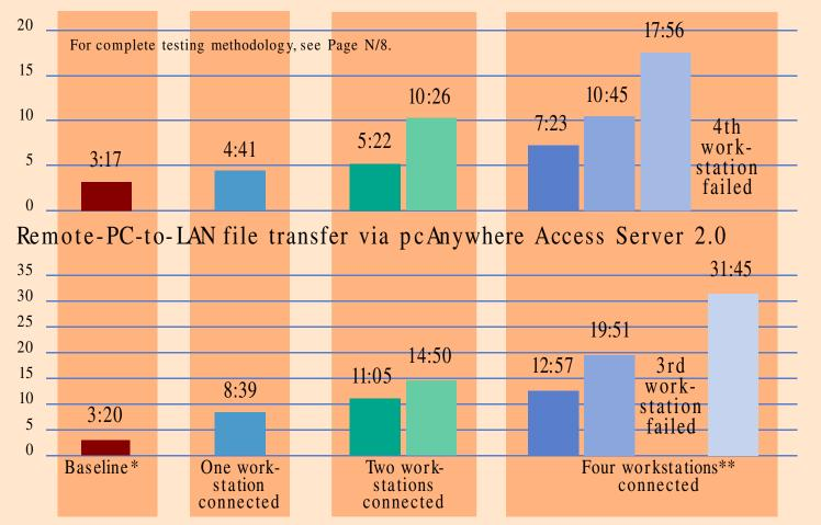
\*As a baseline in the LAN-to-remote-PC test, we transferred the file set from the network drive of our host pcAnywhere client to the hard drive of our local pcAnywhere client. For the remote-PC-to-LAN baseline, we transferred the file set from our local client to the host client's mapped network drive. \*\*Only three out of the four workstations completed the test.
