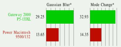
Both computers were equipped with an ATITechnologies Inc. Mach64-based graphics accelerator card. Both computers were equipped with 65M bytes of system RAM so that each test could be run entirely in system memory. This eliminated the effects of hard-disk access on performance.
