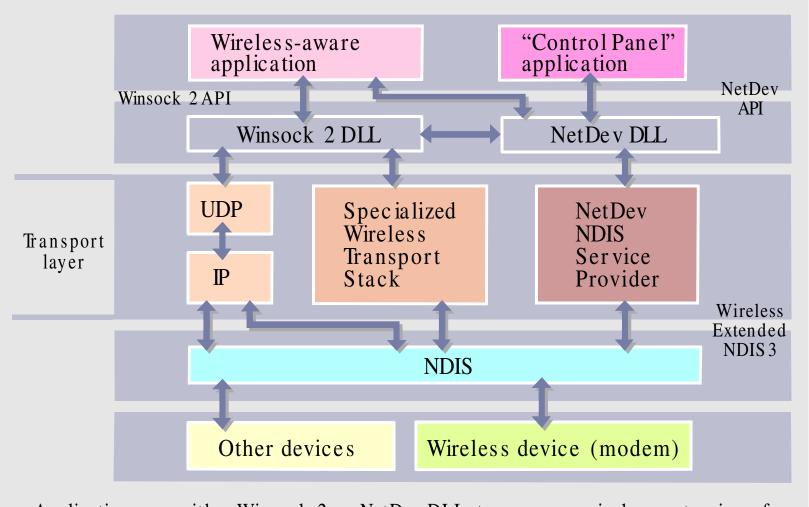
Applications use either Winsock 2 or NetDev DLLs to access a wireless extension of NDIS, which in turn provides the interface to wireless modems or other devices.
