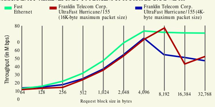
Our test LAN consisted of five EISA workstations and a NetWare 3.12 file server, each equipped with a Hurricane/155 NIC and daisy-chained via the Hurricane/155's built-inhub port to provide LAN connectivity. To represent the Fast Ethernet camp, we used NetWorth Inc.'s SwiftNIC 10/100TX EISA adapter with Asante Technologies Inc.'s AsanteFast 100 Hub as a repeater. We measured the results using NetBench 3.01's NIC Throughput test.
