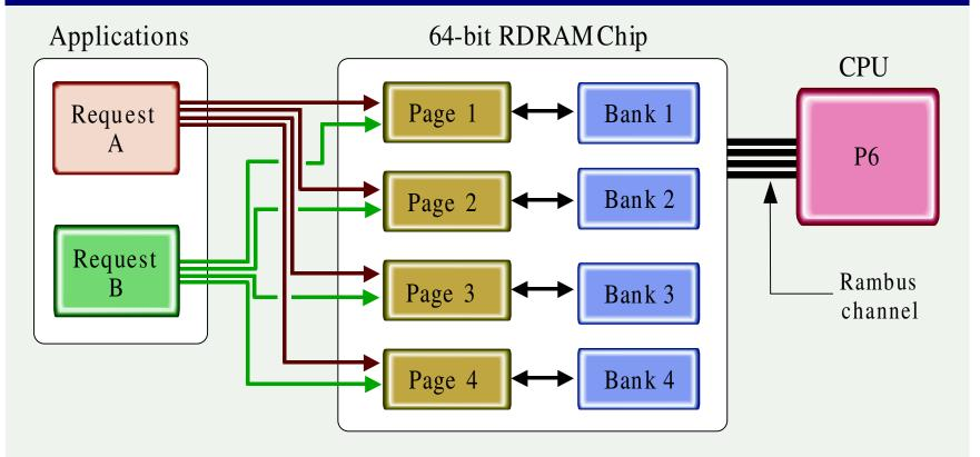
Via its high-speed multiple-bank architecture, the chip can handle up to four outstanding memory instructions at once, which enable users to perform more than one operation at a time.
