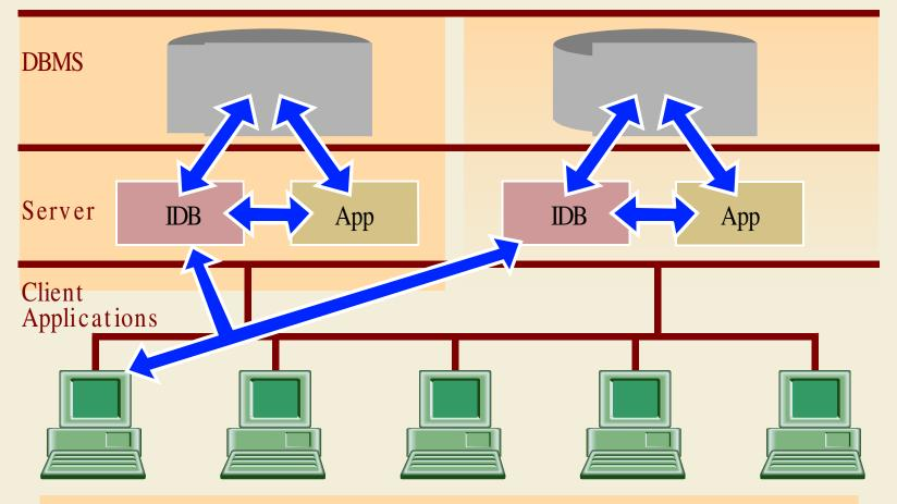
Isis for Database runs in tandem with online replicated database applications to ensure continuous operation.
