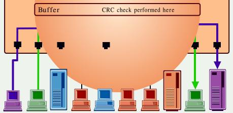
With store-andforward technology, the entire packet is received, checked for errors, then forwarded to the destination address.
