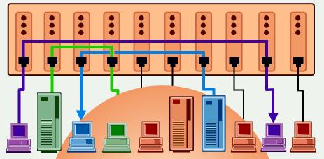
With the cutthrough switching scheme, the packet is transferred to the receiving port as soon as the address can be determined.
