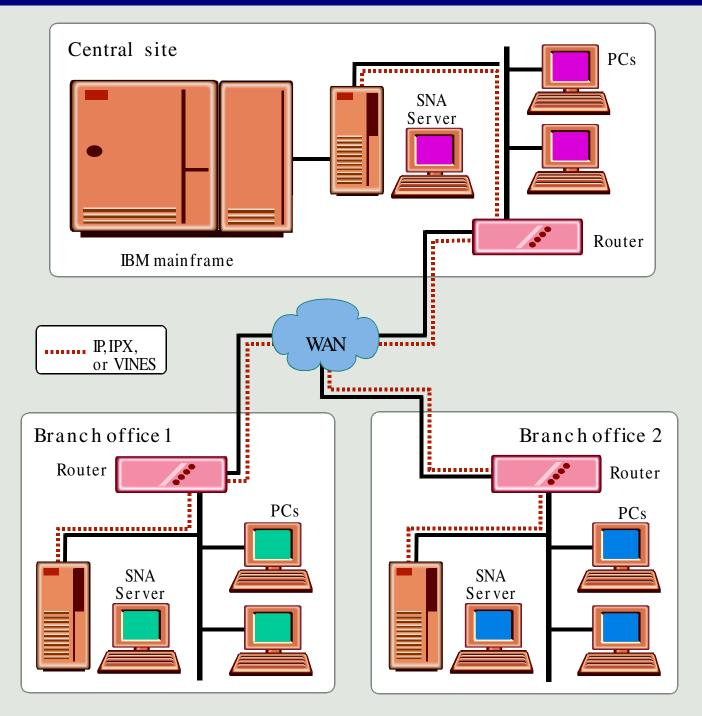
Microsoft's new distributed gateway service for SNA Server for NT allows branch offices to access central-site hosts using existing LAN protocols. SNA Servers at the central site take the traffic destined for the host and strip off the LAN protocols so that only SNA traffic goes into the host.
