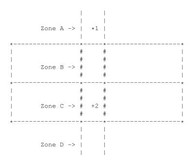
In the diagram point 2 (+) is a blue (upper zone control point), and point 1 (\*) is a pink, lower zone control point. Zones B and C comprise a gantry above a large room, whilst zones A and D are corridors leading out onto that gantry. As you can see, given the arrangement above, the upper part of zone C and the lower part of zone D should BOTH be linked to point 2, and the lower part of zone A and the upper part of zone B should both be connected to point 1.
