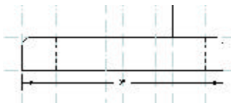
Positioning the dimension line
