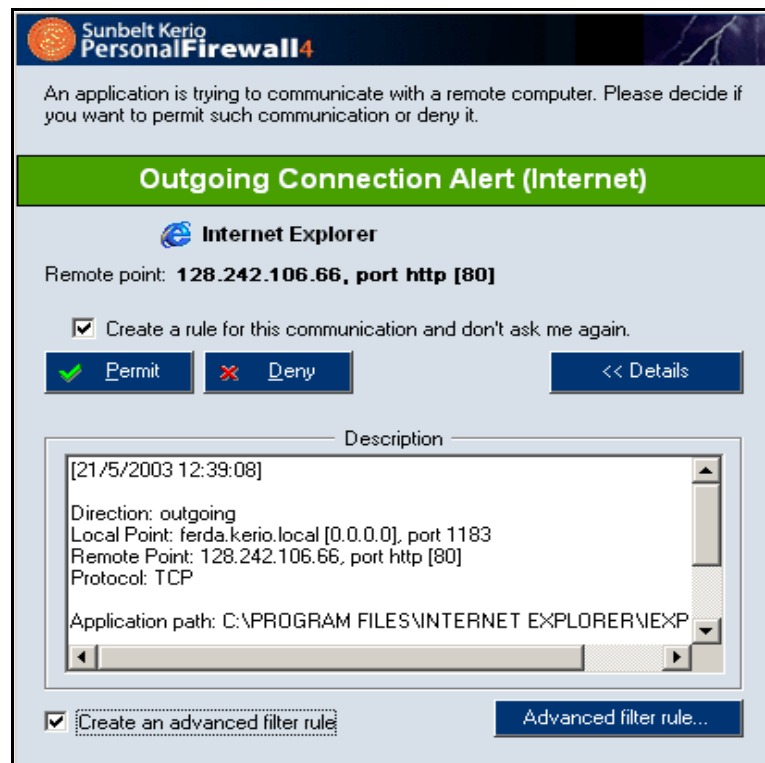
Figure 5-1 Connection alert (unknown traffic detection)
