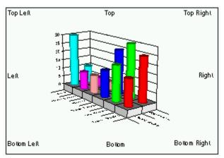
Width To Height and Depth To Height. Enter a positive number in each of these fields to represent the percentage of the charts height used to draw the charts width and depth.
