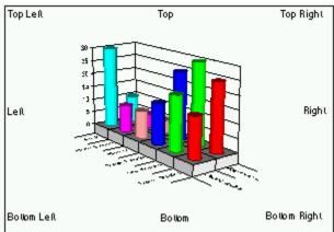
Ambient Light. This type of light shines on all sides of chart elements and is cast in addition to light from fixed light sources. If ambient light is set to 100 percent, all sides of the chart elements are illuminated equally no matter what light sources you turn on. If ambient light is set to 0, only the sides of chart elements facing the active light sources are illuminated.
