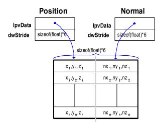
In this case, the **lpvData** members of the **D3DDP\_PTRSTRIDE** structures point to two locations within the same buffer, and the strides are set to the combined width of the interleaved components. Of course, you aren't limited to any particular interleaving scheme. So long as you set the data pointers and their strides correctly, any interleaving scheme will work.
