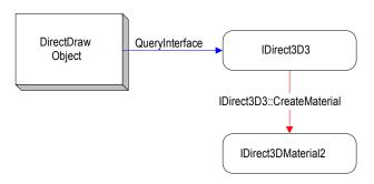
You create a material by calling the **IDirect3D3::CreateMaterial** method. The first parameter is the address of the variable that will contain a valid **IDirect3DMaterial3** interface pointer if the call succeeds. The method's second
