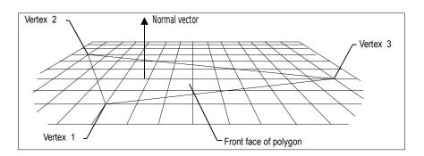
Any face that is not a front face is a back face. Direct3D does not always render back faces, therefore back faces are said to be culled. (You can change the culling mode to render back faces, if so desired. See Culling State for more information.)
