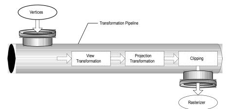
At the head of the pipeline, no transformations have been applied, so all of a model's vertices are declared relative to a local coordinate system (this is a local origin and an orientation). This orientation of coordinates is often referred to as model space, and individual coordinates are called model coordinates.
