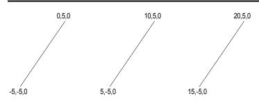
You can apply materials and textures to a line list. The colors in the material or texture only appear along the lines drawn, not at any point in between the lines.
