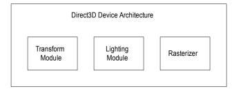
Direct3D enables applications that utilize custom transformation and lighting models to bypass the Direct3D device's transformation and lighting modules. For details, see Vertex Formats.
