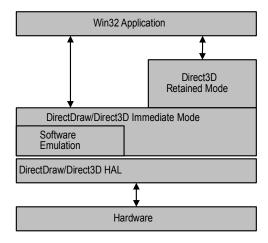
Direct3D is tightly integrated with the DirectDraw component of DirectX®. DirectDraw surfaces are used as rendering targets (front and back surfaces) and as zbuffers. The Direct3D COM interface is actually an interface to a DirectDraw object.
