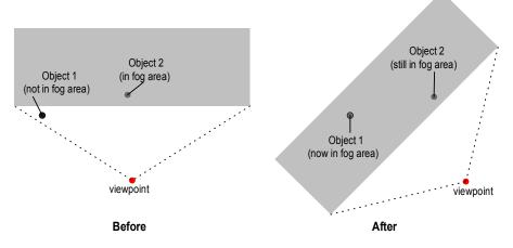
Range-based fog is another, more accurate, way to determine the fog effects. In range-based fog, Direct3D uses the actual distance from the viewpoint to a vertex for its fog calculations, increasing the effects of fog as the distance between the two points increases, rather than the depth of the vertex within in the scene, thereby avoiding rotational artifacts.
