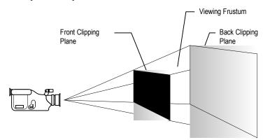
If you imagine that you are standing in a dark room and looking out through a square window, you are visualizing a viewing frustum. In this analogy, the near-clipping plane is the window, and the back clipping plane is whatever finally interrupts your view—the skyscraper across the street, the mountains in the distance, or nothing at all. You can see everything inside the truncated pyramid that starts at the window and ends with whatever interrupts your view, and you can see nothing else.
