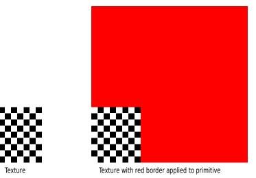
How your application sets the border color depends on what version of the Direct3D device interface it uses. If your application uses the **IDirect3DDevice3** interface, set the border color by calling **IDirect3DDevice3::SetTextureStageState**. Set the first parameter for the call to the desired texture stage identifier, the second parameter to
