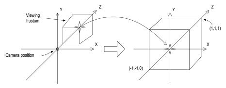
In the perspective transformation, the limits of the x- and y-directions are -1 and 1. The limits of the z-direction are 0 for the front plane and 1 for the back plane.
