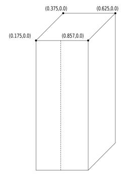
With wrapping enabled in the U direction, the textured pillar shows the colors and symbols from the environment map appropriately and, at the "seam" in the front of the texture, the rasterizer properly chooses the shortest route between the texture coordinates, assuming that U coordinates 0.0 and 1.0 share the same location. The textured pillar would look something like the following:
