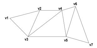
The system uses vertices v1, v2, and v3 to draw the first triangle, v2, v4, and v3 to draw the second triangle, v3, v4, and v5 to draw the third, v4, v6, and v5 to draw the fourth, and so on. Notice that the vertices of the second and fourth triangles are out of order; this is required to make sure that all of the triangles are drawn in a clockwise orientation.
