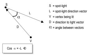
Next, the system compares this value to the cosine of the spot light's inner and outer cone angles. In the light's **D3DLIGHT2** structure, the **dvTheta** and **dvPhi** members represent the total cone angles for the inner and outer cones. Because the attenuation occurs as the vertex becomes more distant from the center of illumination, rather than across the total cone angle, Direct3D halves these cone angles before calculating their cosines.
