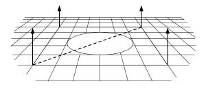
In this case, the Gouraud shade mode, which interpolates between vertices, would miss the spotlight altogether; the face would be rendered as though the spotlight did not exist.
