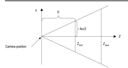
In this illustration, the variable D is the distance from the camera to the origin of the space that was defined in the last part of the geometry pipeline—the viewing transformation. This is the space around which you arrange the limits of your viewing frustum. For information about how this D variable is used to build the projection matrix, see What Is the Projection Transformation?
