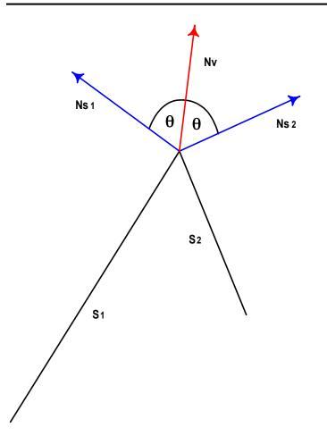
If the vertex normal leans toward one of the faces with which it is associated, it causes the light intensity to increase or decrease for points on that surface, depending on the angle it makes with the light source. An example is shown in the following figure. Again, these surfaces are seen edge-on. The vertex normal leans toward S1, causing it to have a smaller angle with the light source than it would if the vertex normal had equal angles with the surface normals.
