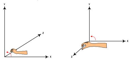
Direct3D uses a left-handed coordinate system. If you are porting an application that relies on right-handedness, you can do so by making two simple changes to the data passed to Direct3D.
