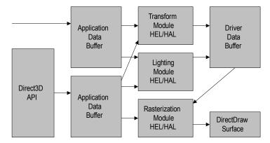
You can disable the lighting module or both the lighting and transformation when you are working with execute buffers. This changes the way the vertex list is interpreted, allowing the user to supply pretransformed or prelit vertices only for the rasterization phase of the rendering pipeline. Note that only one vertex type can be used in each execute buffer. For more information about vertex types, see Vertex Formats.
