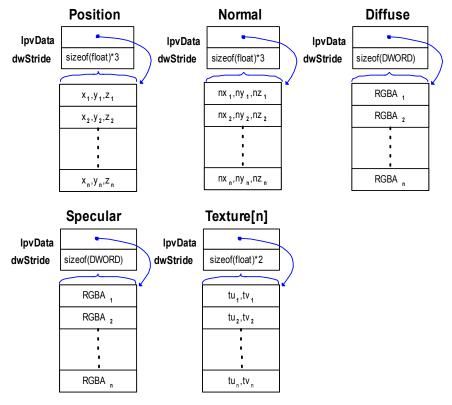
to arrange vertex components however it needs. For instance, you might use distinct arrays for every vertex component, as shown in the following illustration.
