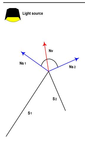
You can use the Gouraud shade mode to display some of the objects in a 3-D scene with sharp edges. If you are using execute buffers, your application needs to duplicate the vertex normal vectors at any intersection of faces where a sharp edge was required, as shown in the following illustration.
