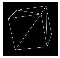
You can also use triangles to create primitives whose surfaces appear to be smooth curves. The following illustration shows how a sphere can be simulated with triangles. After a material is applied, it looks curved when it is rendered. This is especially true if using Gouraud shading. For details, see Gouraud Shading
