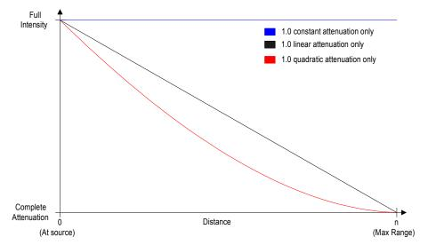
Note that using only quadratic attenuation often results in harsh transition between light and dark over distance. Each of the curves uses only one of the attenuation factors, but you are free to mix these values to create different attenuation effects.
