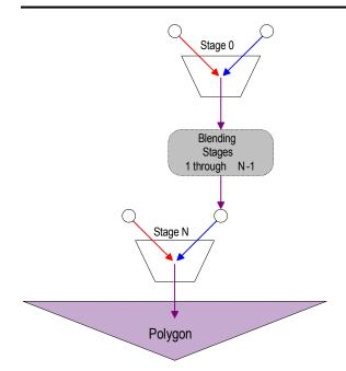
Each stage in a device has a zero-based index. Direct3D for DirectX 6.0 allows up to eight blending stages, although you should always check device capabilities to determine how many stages the current hardware supports. The first blending stage is at index 0, the second is at 1, and so on up to index 7. The system blends stages in increasing order of index.
