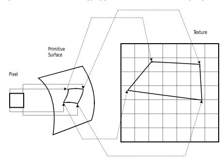
For this example, we are idealizing a pixel, shown at the left of the illustration, into a square of color. The addresses of the four corners of the pixel are mapped onto the 3-D primitive in object space. The shape of the pixel is often distorted because of the shape of the primitive in 3-D space and because of the viewing angle. The corners of the surface area on the primitive that correspond the corners of the pixel are then
