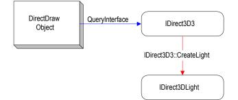
You create a light object by calling the **IDirect3D3::CreateLight** method. The first parameter is the address of a variable that will contain a valid **IDirect3DLight** interface pointer if the call succeeds. The method's second parameter is intended to be used in COM aggregation — because aggregation is not implemented, this parameter must be set to NULL. The following example shows what the code to make this call might look like:
