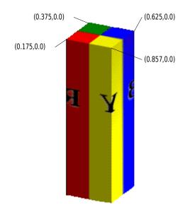
If texture wrapping wasn't enabled, the rasterizer would not interpolate in the direction needed to generate a believable, reflected, image. Rather, the area at the front of the pillar would contain a horizontally compressed version of the texels between U coordinates 0.175 and 0.875, as they pass through the center of the texture. The effect would be ruined.
