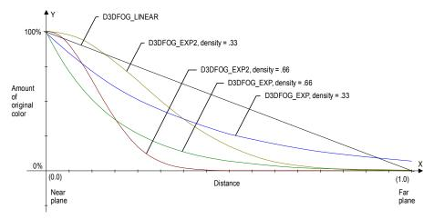
When Direct3D calculates fog effects, it uses the fog factor from one of the preceding equations in a blending formula, shown here:
