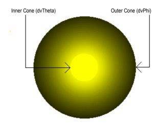
Spotlights are affected by falloff, attenuation, and range. These factors, as well as the distance light travels to each vertex, are figured in while computing lighting effects for objects in a scene. Computing all these effects for each vertex makes spotlights the most computationally expensive of all lights in Direct3D Immediate Mode.
