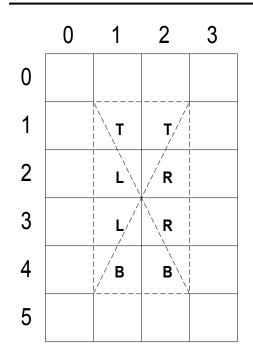
If you move the rectangle in the previous example so that its upper-left corner is at (1.0, 1.0), its lower-right corner at (3.0, 5.0), and its center point at (2.0, 3.0), Direct3D applies the top-left filling convention. Most of the pixels in this rectangle would straddle the border between two or more triangles, as the next illustration shows.
