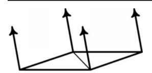
It is more likely, however, that your object is made up of triangle strips, and that the triangles are not coplanar. One simple way to get smooth shading across all of the triangles in the strip is to first calculate the surface normal vector for each polygonal face with which the vertex is associated. The vertex normal can be set to make an equal angle with each of the surface normals. Note, however, that this method may not be efficient enough for complex primitives.
