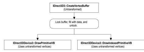
As shown in the preceding illustration, the **IDirect3DDevice3::DrawPrimitiveVB** and **IDirect3DDevice3::DrawIndexedPrimitiveVB** methods are capable of rendering from a non-transformed vertex buffer. In this case, the system performs vertex and rendering operations each time you call a rendering method. For DirectX
