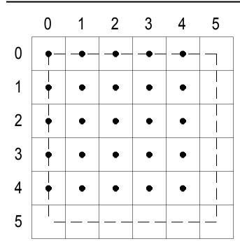
In the top-left filling convention, the word "top" refers to the vertical location of horizontal spans, and the word "left" refers to the horizontal location of pixels within a span. An edge cannot be a top edge unless it is horizontal—in the general case, most triangles will have only left and right edges.
