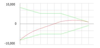
Note that during the sustain portion of the envelope, the magnitude of the effect follows the same straight line as before the envelope was applied. For the duration of the attack and fade, the slope of the ramp is modified by the attack and fade levels.
