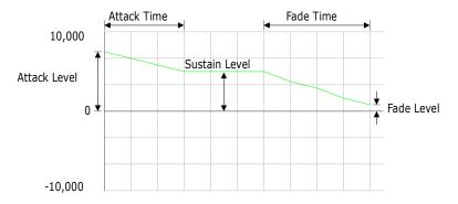
The next diagram shows the result of the envelope being applied to the periodic effect in the first diagram. Note that the envelope is mirrored on the negative side of the magnitude. An attack value of 8,000 means that the initial magnitude of the force in either direction will be 80 percent of the maximum possible.
