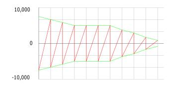
Periodic effects and conditions can also be modified by the addition of an *offset*, which defines the amount by which the waveform is shifted up or down from the base level. The practical effect of applying a positive offset to the sawtooth example would be to strengthen the positive force and weaken the negative one — in other words, the force would peak more strongly in one direction than in the other.
