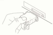
**3** Plug the 3-D SPEX into the glasses jack on the back of the parallel port interface.
