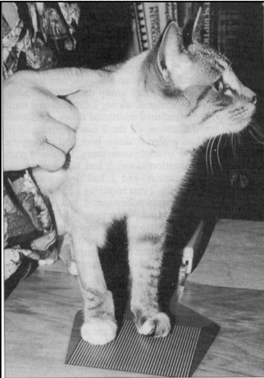
Figure 1—Photograph of a cat standing on a pressure-sensitive mat for measurement of force applied by the forelimbs.
