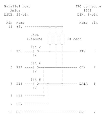
The 7406 (a 74LS05 will do as well) must be connected to +5V and GND of course. The trained technician will notice that this is the same circuit found inside the real C64.
