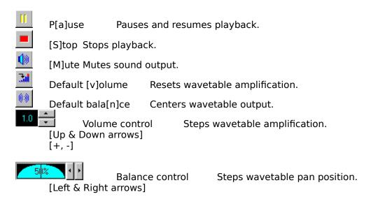
The volume and balance controls do not take effect immediately. The sound data already pipelined for playback - typically some ten seconds of it - has to get out of the way first.
